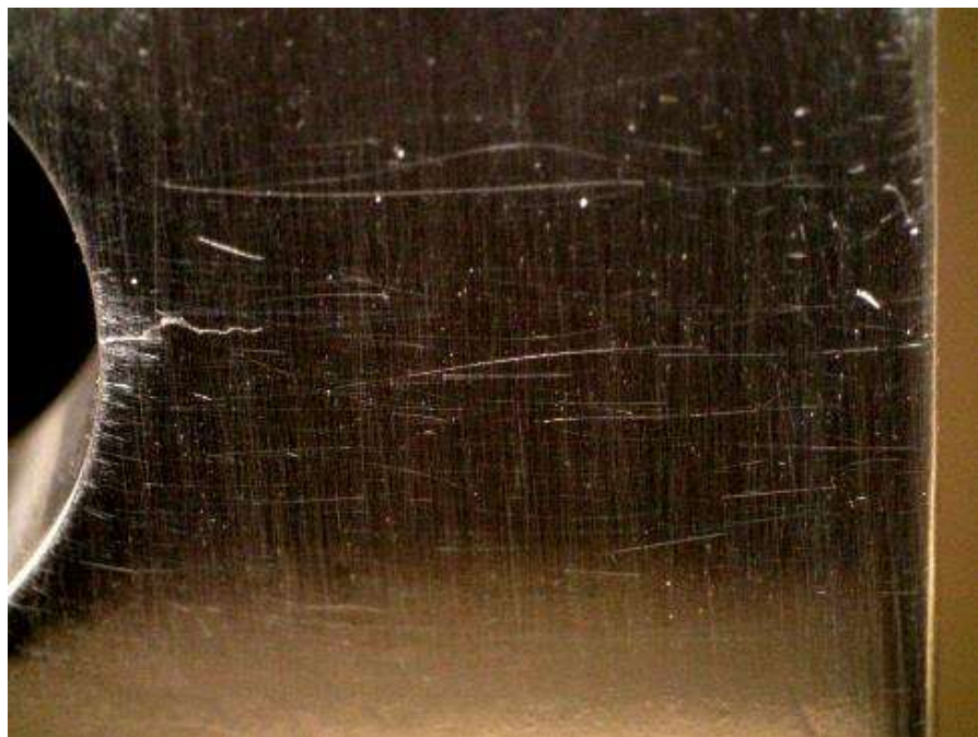
Figure E.29: Specimen CX150ED-3 under 19.8 ksi applied stress. Crack is approximately 0.102 inches in length and appears to be open.
