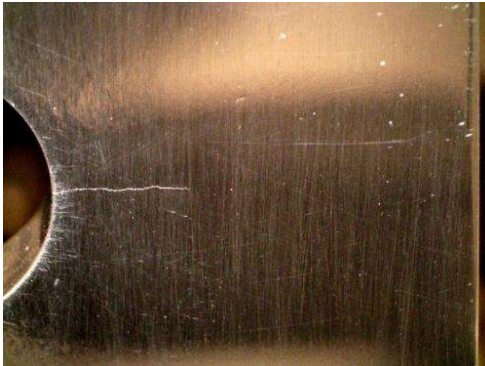
Figure 2.8: Crack growth image captured with USB digital microscope.
