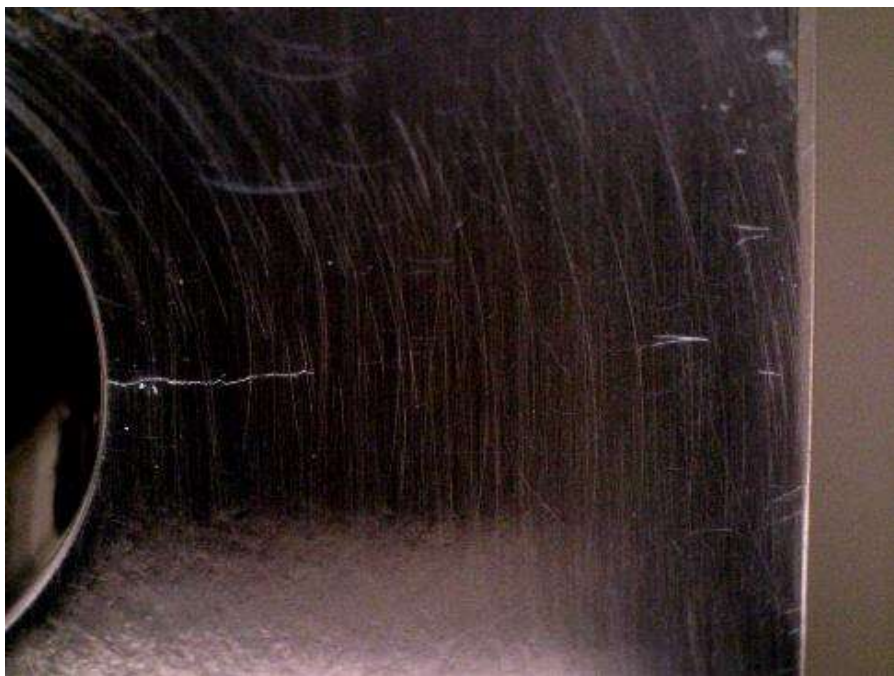
Figure E.16: Specimen CX140ED-2 under 13.2 ksi applied stress. Crack is approximately 0.140 inches in length and appears to be open.
