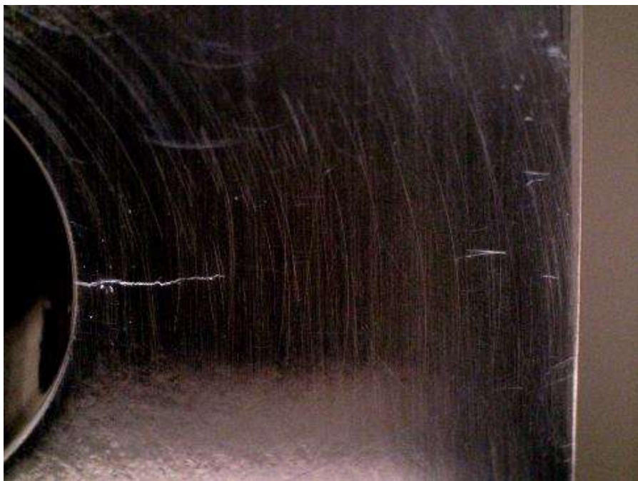
Figure E.19: Specimen CX140ED-2 under 23.1 ksi applied stress. Crack is approximately 0.140 inches in length and appears to be open.
