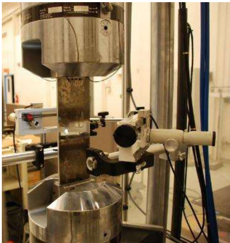
Figure 2.20: Travelling microscope orientation for measuring bore crack length.
