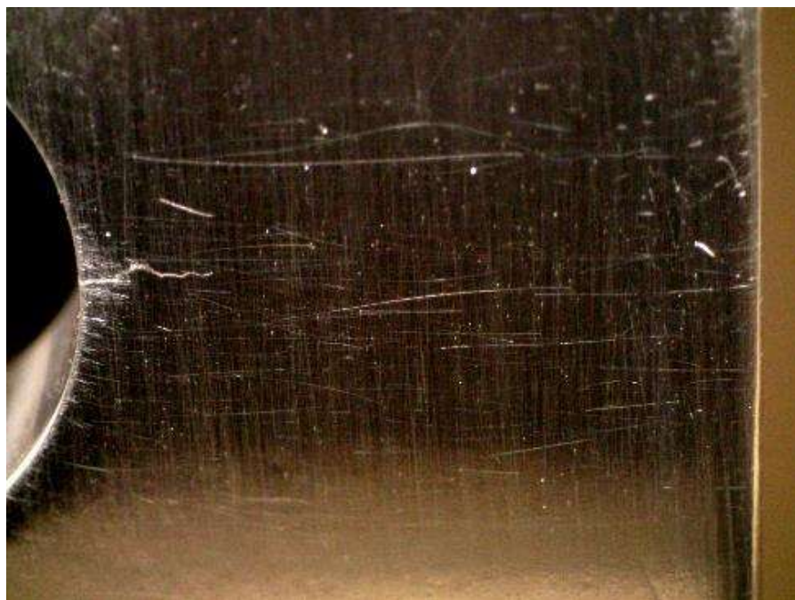
Figure E.30: Specimen CX150ED-3 under 23.1 ksi applied stress. Crack is approximately 0.102 inches in length and appears to be open.
