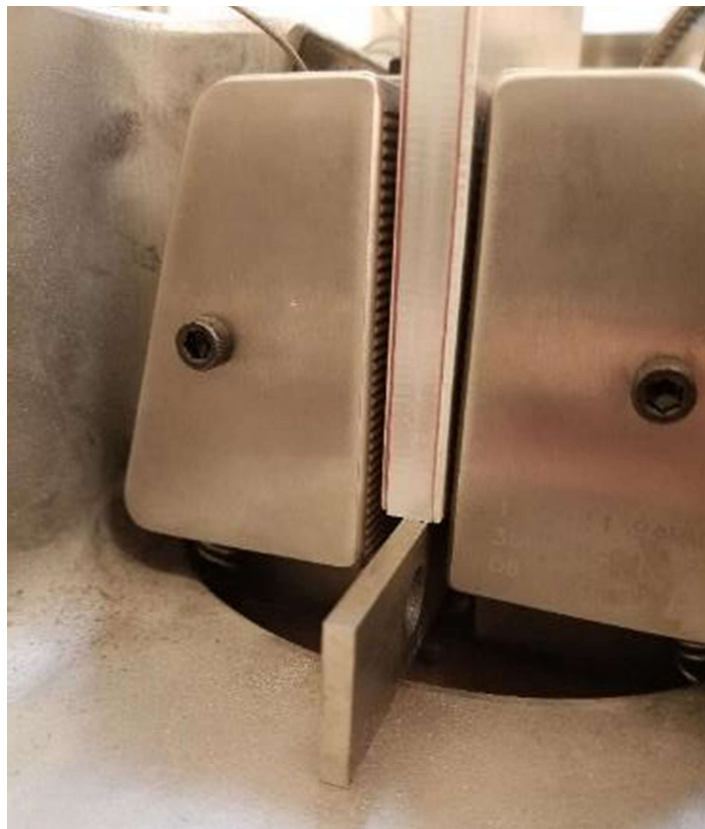
Figure 2.14: Machinist parallel used to align specimen vertically in test machine grips.
