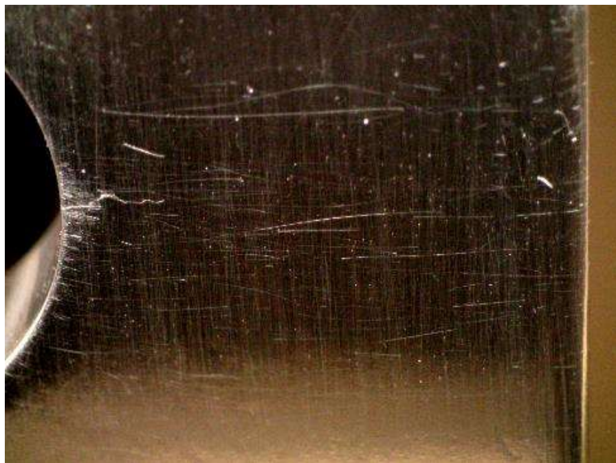
Figure E.27: Specimen CX150ED-3 under 13.2 ksi applied stress. Crack is approximately 0.102 inches in length and appears to be closed.
