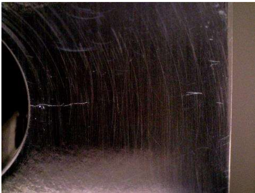
Figure E.13: Specimen CX140ED-2 under 3.3 ksi applied stress. Crack is approximately 0.140 inches in length and appears to be closed.
