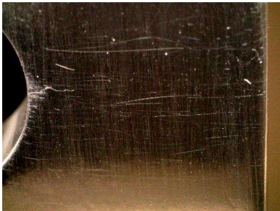
Figure E.26: Specimen CX150ED-3 under 9.9 ksi applied stress. Crack is approximately 0.102 inches in length and appears to be closed.
