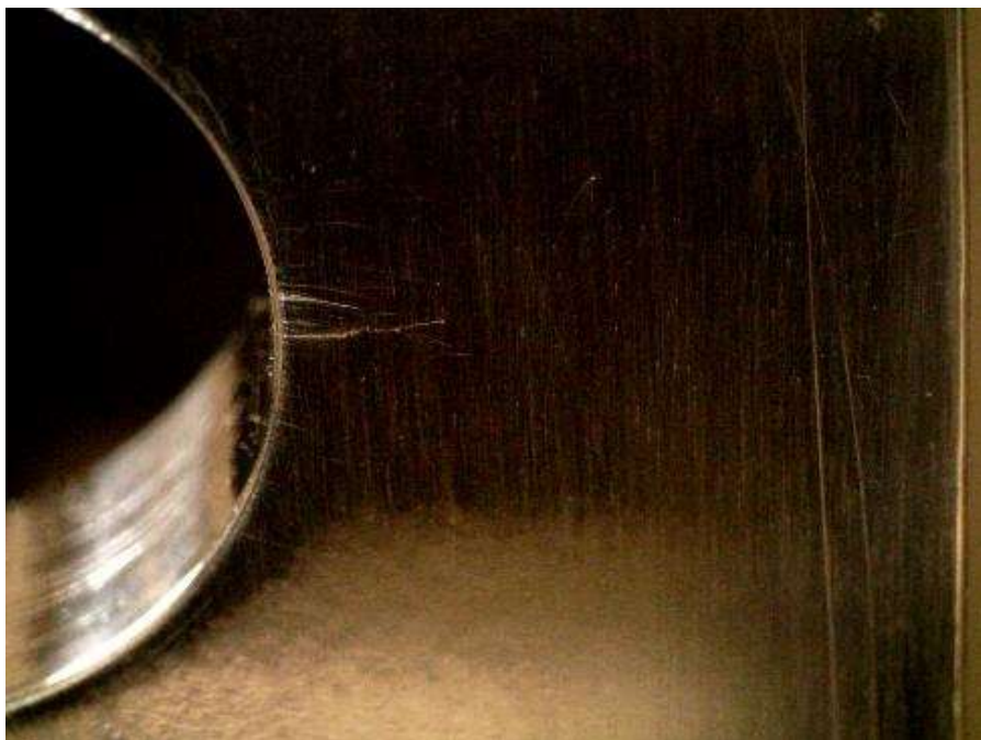
Figure E.1: Specimen CX130ED-2 under zero applied stress. Crack is approximately 0.103 inches in length and appears to be closed.
