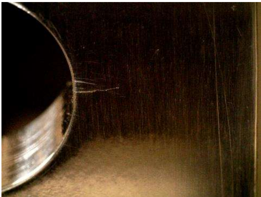
Figure E.3: Specimen CX130ED-2 under 6.6 ksi applied stress. Crack is approximately 0.103 inches in length and appears to be closed.
