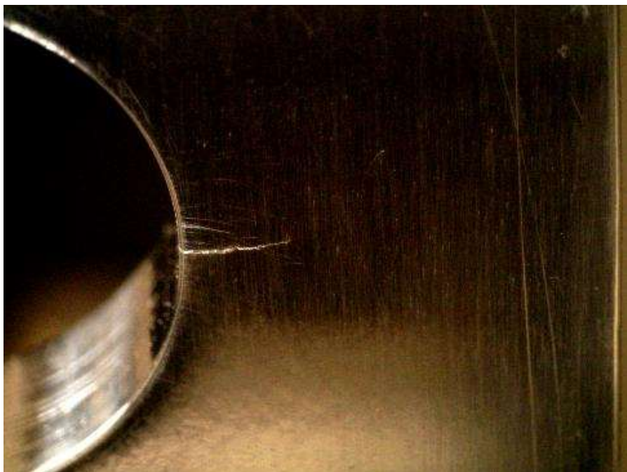
Figure E.11: Specimen CX130ED-2 under 33 ksi applied stress. Crack is approximately 0.103 inches in length and appears to be open.
