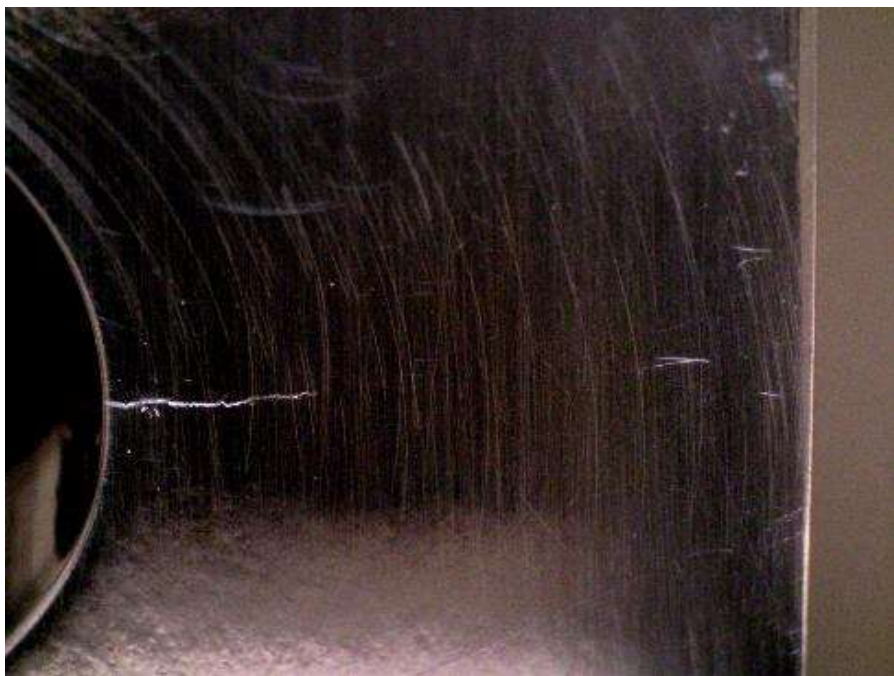
Figure E.20: Specimen CX140ED-2 under 26.4 ksi applied stress. Crack is approximately 0.140 inches in length and appears to be open.
