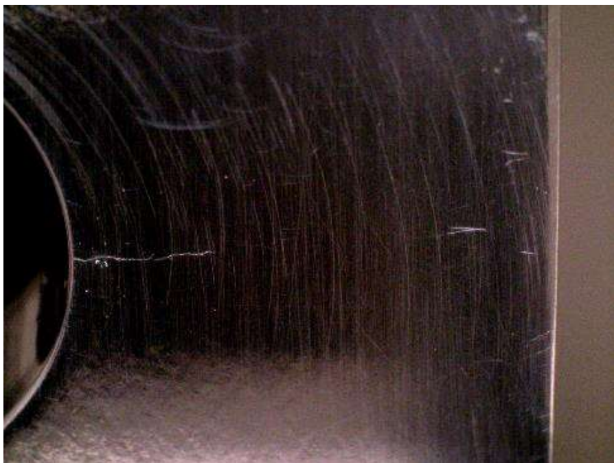
Figure E.15: Specimen CX140ED-2 under 9.9 ksi applied stress. Crack is approximately 0.140 inches in length and appears to be closed.
