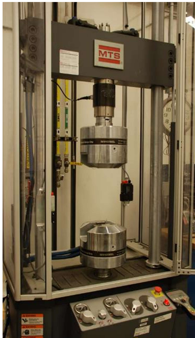
Figure 2.4: Servo-hydraulic load frame used for fatigue testing.
