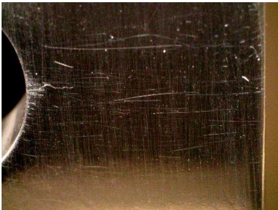
Figure E.24: Specimen CX150ED-3 under 3.3 ksi applied stress. Crack is approximately 0.102 inches in length and appears to be closed.
