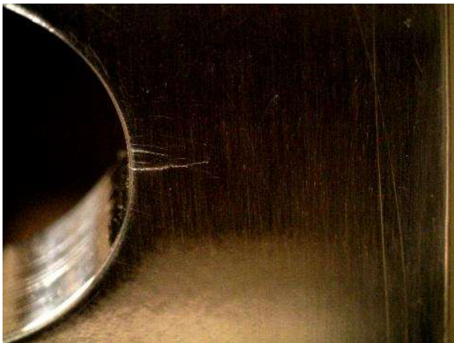
Figure E.7: Specimen CX130ED-2 under 19.8 ksi applied stress. Crack is approximately 0.103 inches in length and appears to be open.
