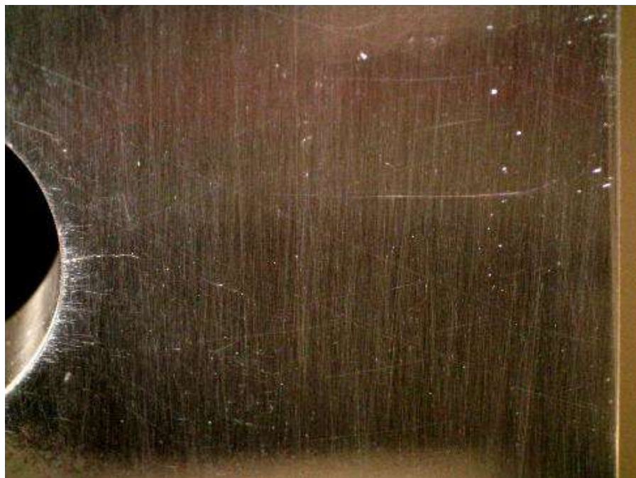
Figure E.41: Specimen CX200ED-3 under 23.1 ksi applied stress. Crack is approximately 0.107 inches in length and appears to be open.
