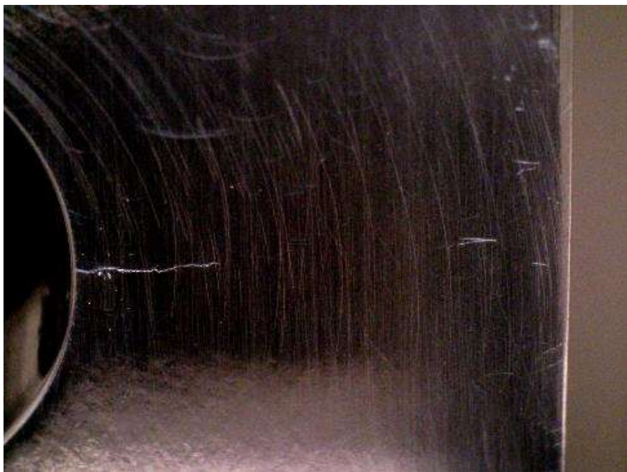
Figure E.17: Specimen CX140ED-2 under 16.5 ksi applied stress. Crack is approximately 0.140 inches in length and appears to be open.
