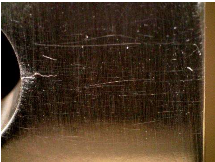
Figure E.31: Specimen CX150ED-3 under 26.4 ksi applied stress. Crack is approximately 0.102 inches in length and appears to be open.
