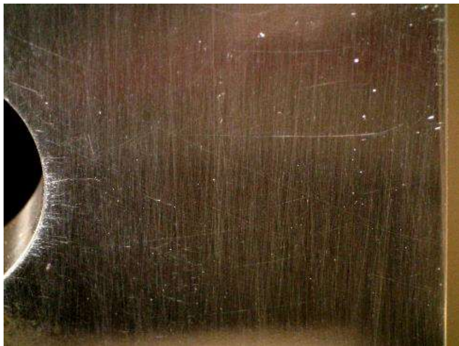
Figure E.38: Specimen CX200ED-3 under 13.2 ksi applied stress. Crack is approximately 0.107 inches in length and appears to be closed.
