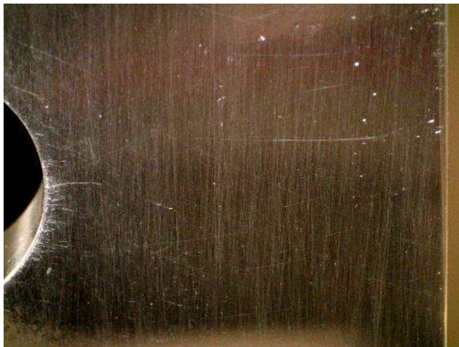
Figure E.40: Specimen CX200ED-3 under 19.8 ksi applied stress. Crack is approximately 0.107 inches in length and appears to be open.
