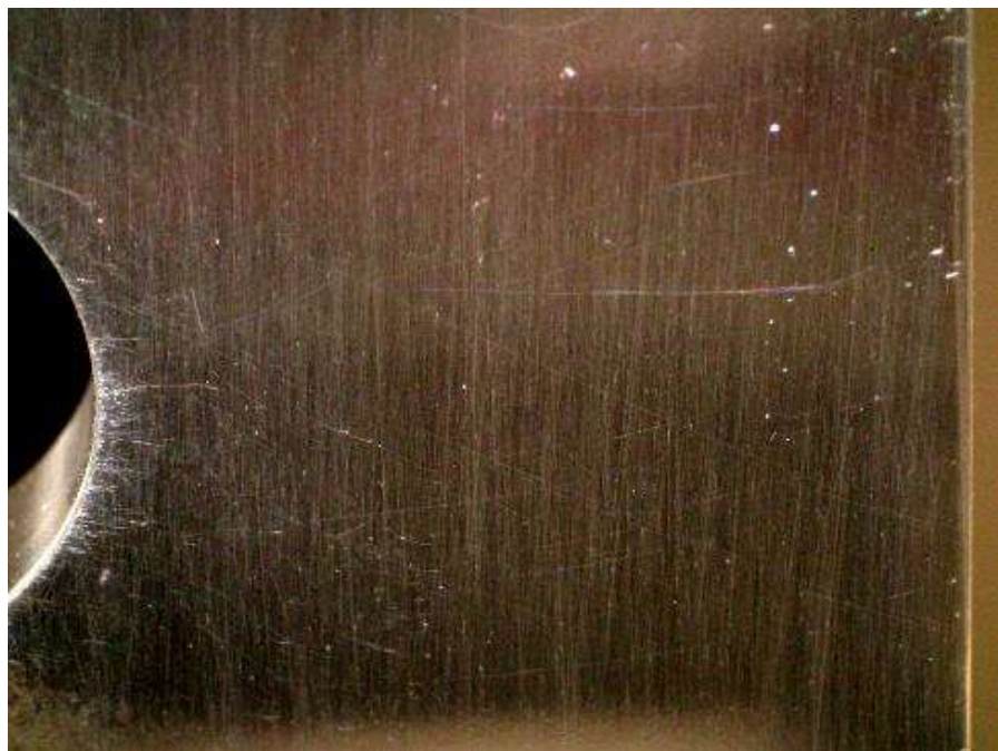
Figure E.37 : Specimen CX200ED-3 under 9.9 ksi applied stress. Crack is approximately 0.107 inches in length and appears to be closed.
