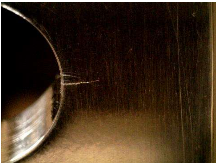
Figure E.9: Specimen CX130ED-2 under 26.4 ksi applied stress. Crack is approximately 0.103 inches in length and appears to be open.
