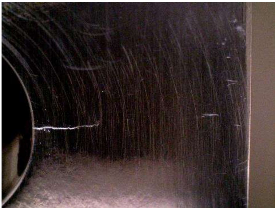
Figure E.22: Specimen CX140ED-2 under 33 ksi applied stress. Crack is approximately 0.140 inches in length and appears to be open.
