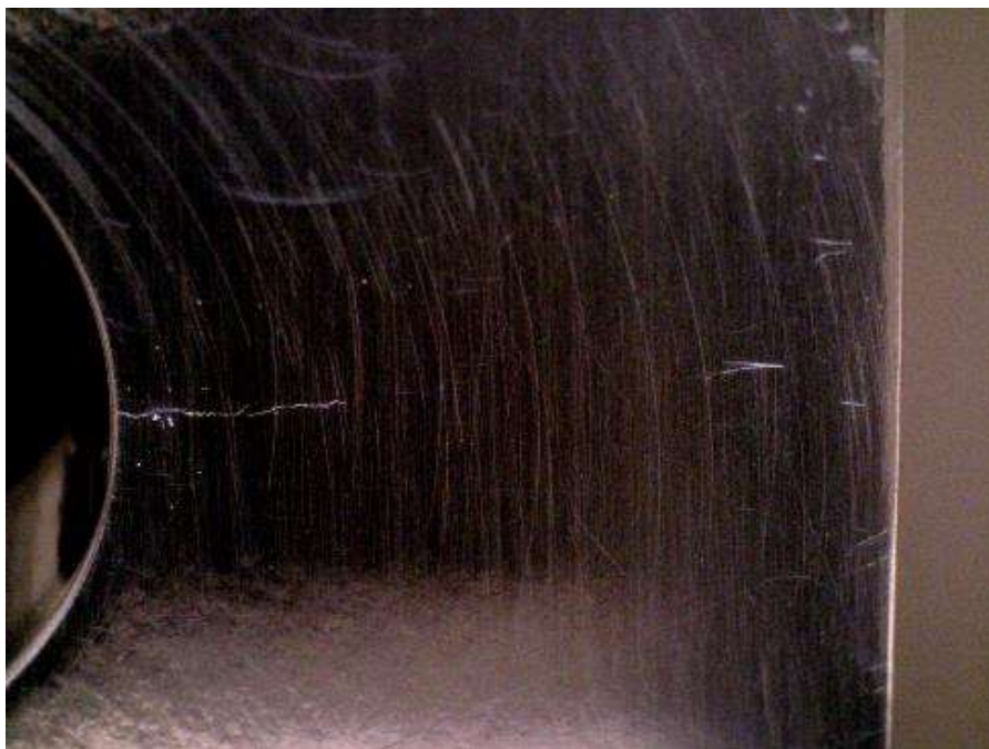
Figure E.14: Specimen CX140ED-2 under 6.6 ksi applied stress. Crack is approximately 0.140 inches in length and appears to be closed.
