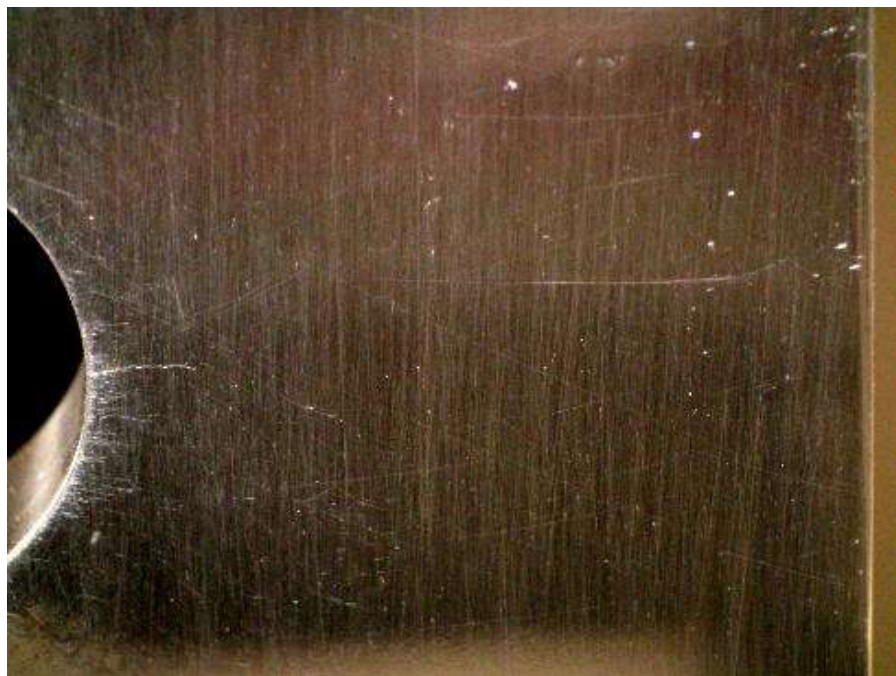
Figure E.42: Specimen CX200ED-3 under 26.4 ksi applied stress. Crack is approximately 0.107 inches in length and appears to be open.
