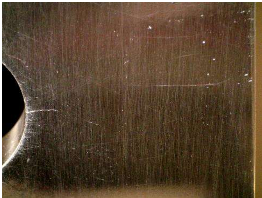
Figure E.44: Specimen CX200ED-3 under 33 ksi applied stress. Crack is approximately 0.107 inches in length and appears to be open.
