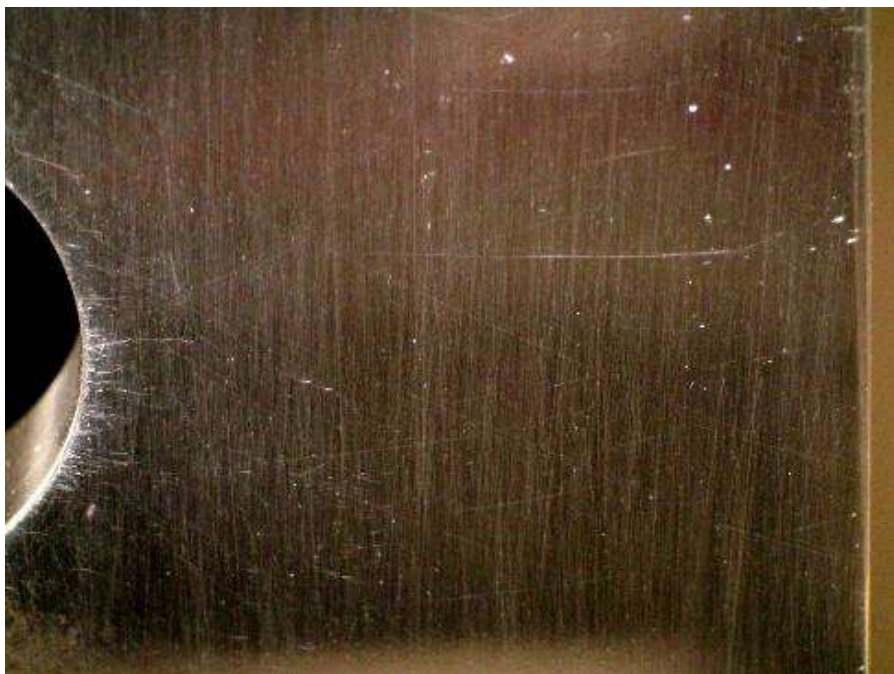
Figure E.35: Specimen CX200ED-3 under 3.3 ksi applied stress. Crack is approximately 0.107 inches in length and appears to be closed.
