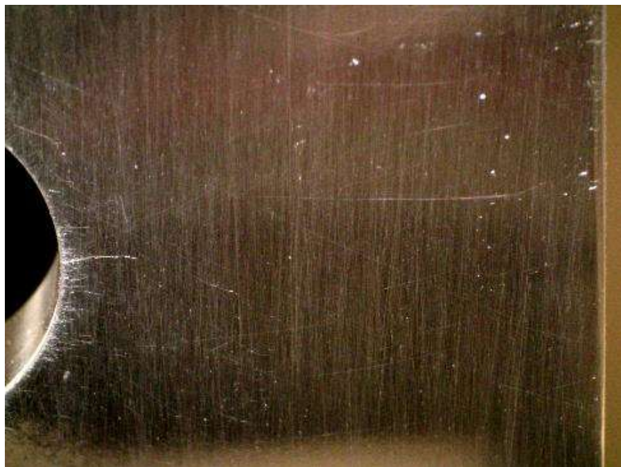
Figure E.43: Specimen CX200ED-3 under 29.7 ksi applied stress. Crack is approximately 0.107 inches in length and appears to be open.
