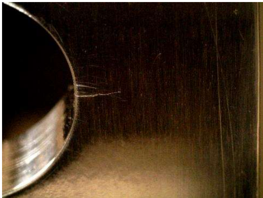
Figure E.6: Specimen CX130ED-2 under 16.5 ksi applied stress. Crack is approximately 0.103 inches in length and appears to be open.
