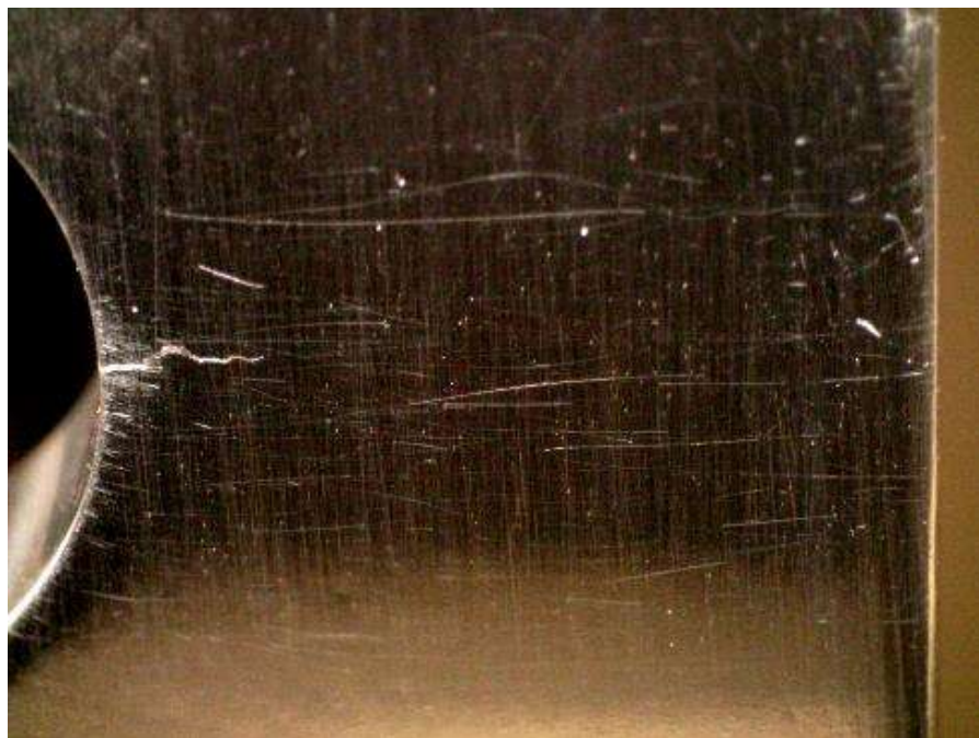
Figure E.33: Specimen CX150ED-3 under 33 ksi applied stress. Crack is approximately 0.102 inches in length and appears to be open.
