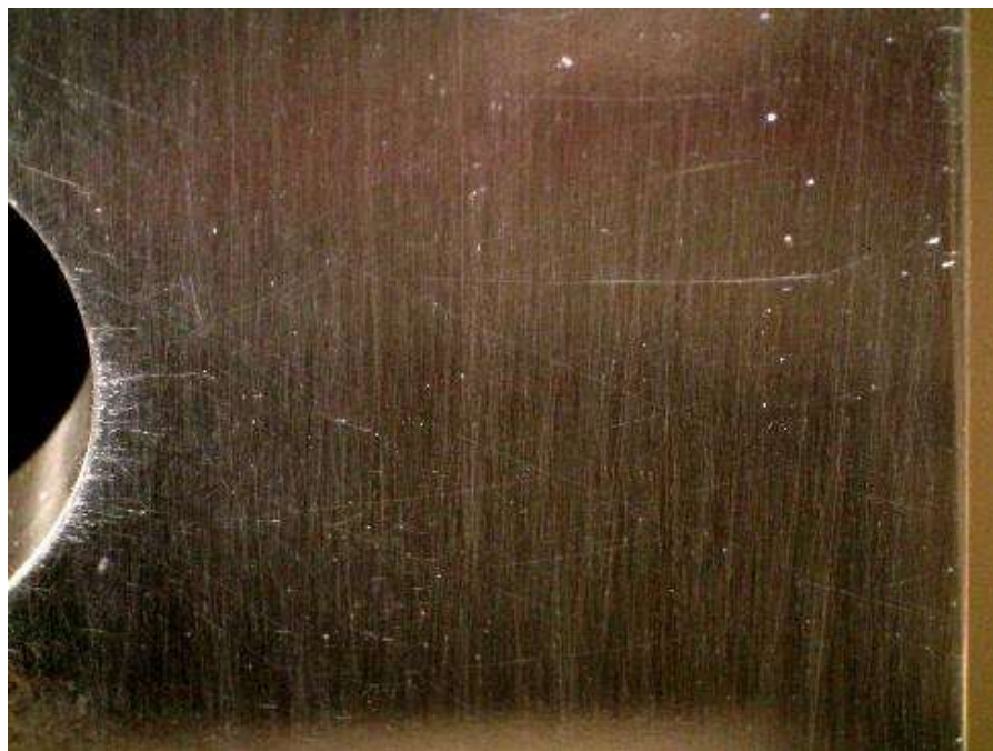
Figure E.34: Specimen CX200ED-3 under zero applied stress. Crack is approximately 0.107 inches in length and appears to be closed.
