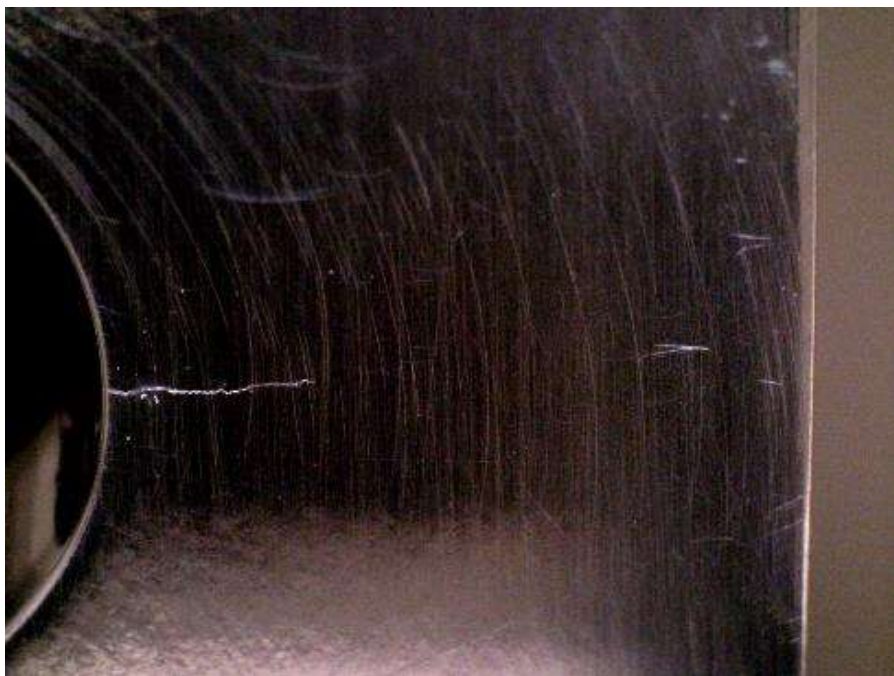
Figure E.18: Specimen CX140ED-2 under 19.8 ksi applied stress. Crack is approximately 0.140 inches in length and appears to be open.
