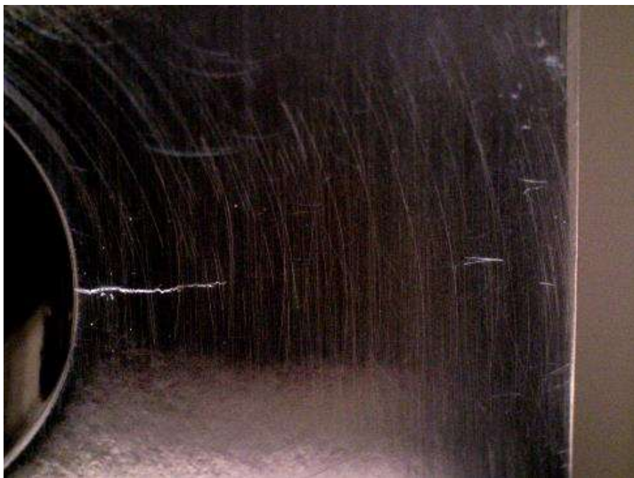
Figure E.21: Specimen CX140ED-2 under 29.7 ksi applied stress. Crack is approximately 0.140 inches in length and appears to be open.
