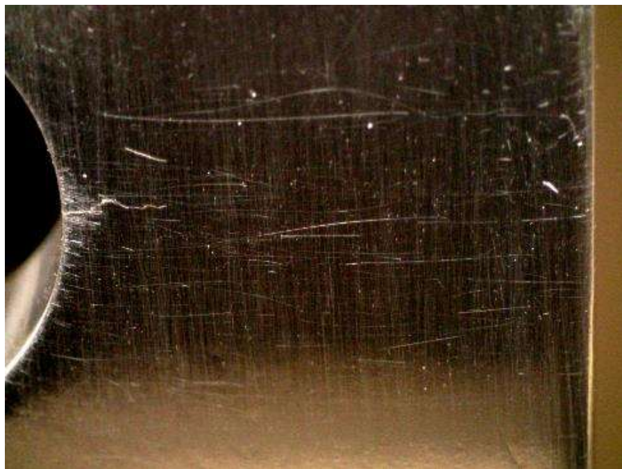
Figure E.28: Specimen CX150ED-3 under 16.5 ksi applied stress. Crack is approximately 0.102 inches in length and appears to be open.
