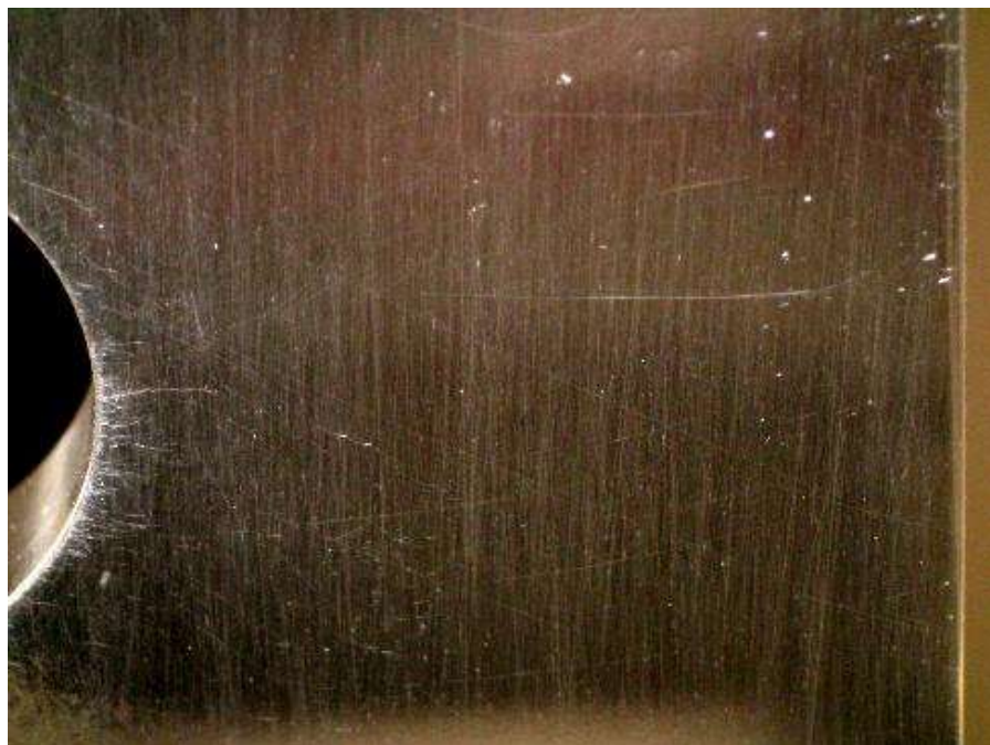
Figure E.39: Specimen CX200ED-3 under 16.5 ksi applied stress. Crack is approximately 0.107 inches in length and appears to be closed.
