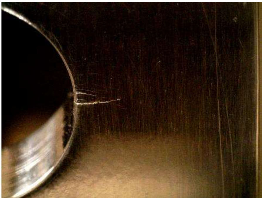
Figure E.10: Specimen CX130ED-2 under 29.7 ksi applied stress. Crack is approximately 0.103 inches in length and appears to be open.
