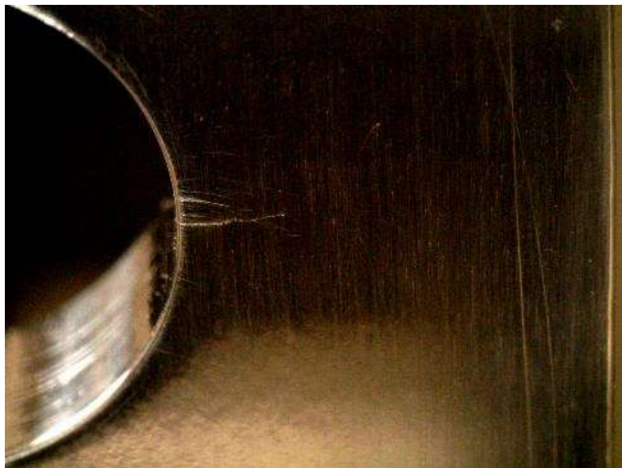
Figure E.5: Specimen CX130ED-2 under 13.2 ksi applied stress. Crack is approximately 0.103 inches in length and appears to be closed.
