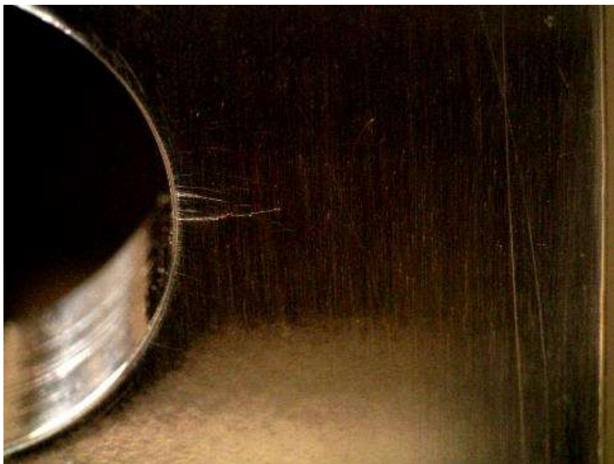
Figure E.4: Specimen CX130ED-2 under 9.9 ksi applied stress. Crack is approximately 0.103 inches in length and appears to be closed.
