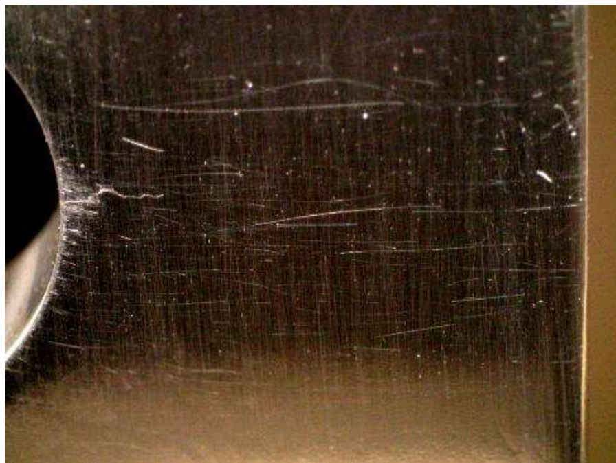
Figure E.25: Specimen CX150ED-3 under 6.6 ksi applied stress. Crack is approximately 0.102 inches in length and appears to be closed.
