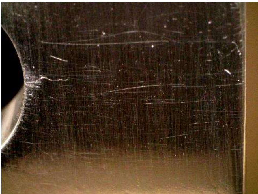
Figure E.23: Specimen CX150ED-3 under zero applied stress. Crack is approximately 0.102 inches in length and appears to be closed.
