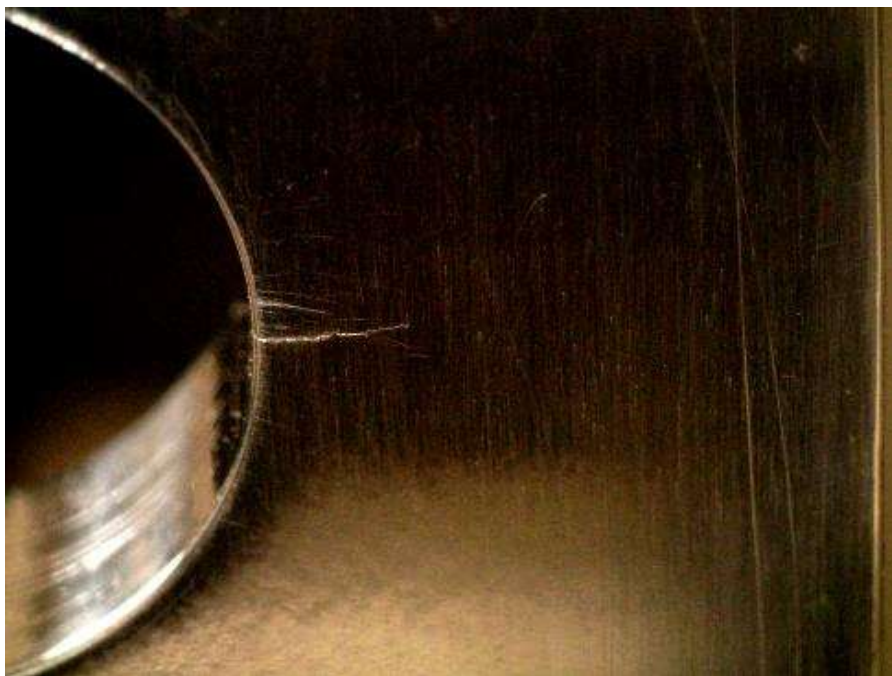
Figure E.8: Specimen CX130ED-2 under 23.1 ksi applied stress. Crack is approximately 0.103 inches in length and appears to be open.
