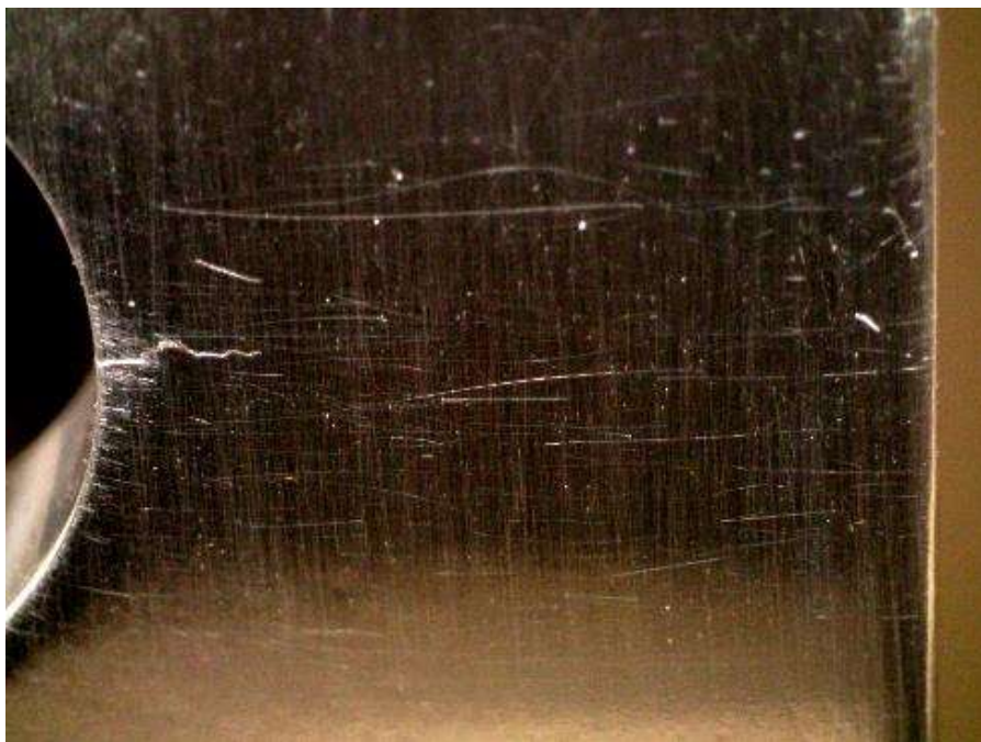
Figure E.32: Specimen CX150ED-3 under 29.7 ksi applied stress. Crack is approximately 0.102 inches in length and appears to be open.
