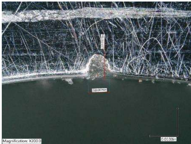
Figure 2.2: Electrical discharge machined (EDM) notch at edge of hole.
